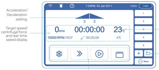
Clear one-touch buttons for fast refrigeration, fast centrifugation, intelligent start-stop and lid-closing status.
