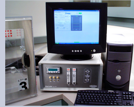
The A410V can use a PC interface (desktop or laptop) to control and monitor oxygen with ease.
