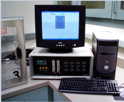
The A84XOV can use a PC interface (desktop or laptop) to control and monitor oxygen with ease.
